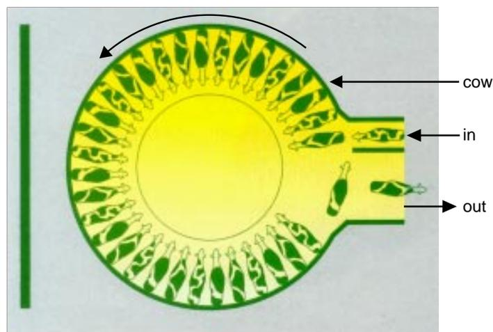
**Figure 3** 32-stall rotary milking shed
