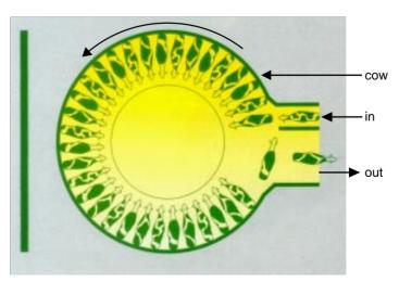
Figure 3 32-stall rotary milking shed
