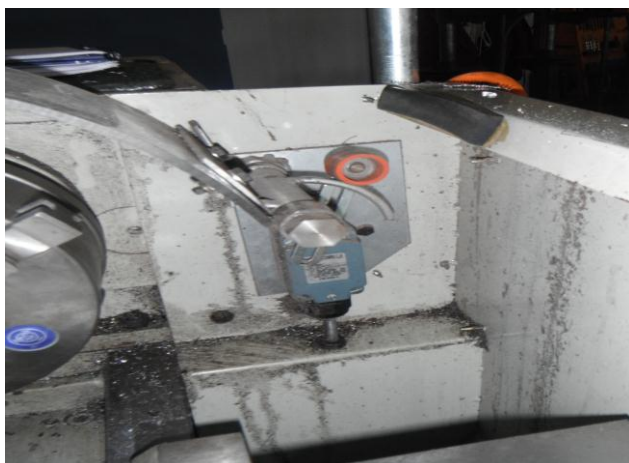
Photo four: side view of chuck guard with interlock
