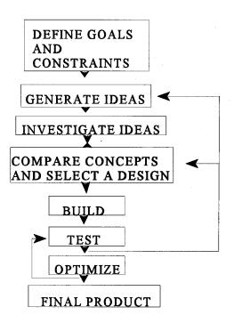
The process presented here may be used at any and all levels of model car design, from the design of individual components to the complete car as a system. The key principle in the process is to start all designs with many ideas, then investigate and evaluate several of them before locking into a design.
